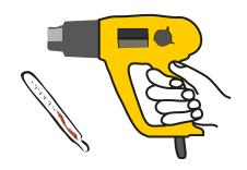
**5.**When the mounting is completed, the vinyl then must be reheated to approx. 95 degrees °C for the vinyl to "forget" its original shape. If the vinyl does not get this afterheat, the vinyl will slowly retreat to its original shape.
