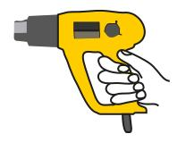
3. In places where the vinyl must be pulled over the workpiece, heat the vinyl with a heat gun to make the vinyl flexible. When the vinyl is heated, it is easy to carefully shape it/pull it over the place/item. IF THE VINYL BECOMES STRETCHED TOO MUCH, YOU CAN RECREATE THE ORIGINAL SHAPE BY HEATING IT UP AGAIN.
